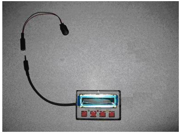
Cable connections for simulation mode (9V battery required)
